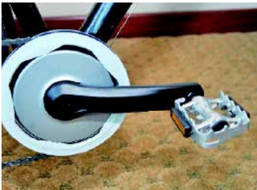
▲SR Suntour's Twinsensor combines torque and rotation sensing points to ensure a smooth start every time.
