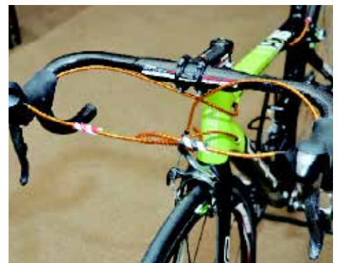
▲ Made of aluminum alloy, the Alligator inlink can be adjusted by angle and length. While riding, the brake and derailleur cables operate smoothly.
