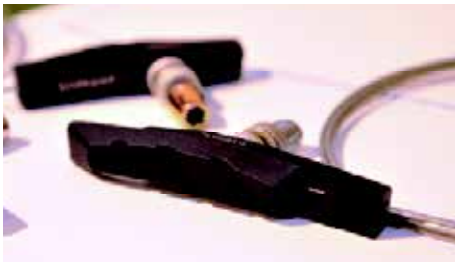
▲ Slidepad is a safety-focused single lever braking technology that reduces the risk of front wheel lock up accidents on bicycles.
