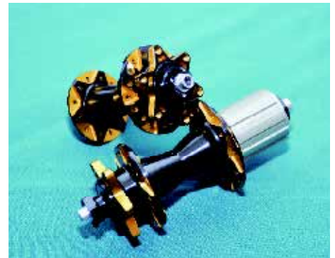
▲ The Rubar RFD MTB hub features a patented axle design, a unique spoke weave and is waterproof. It weighs 340g, not including the quick release set.
