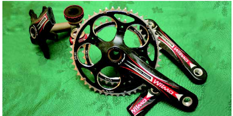
▲ Shun Shing's Wilma hollow crankset weighs only 615g.
