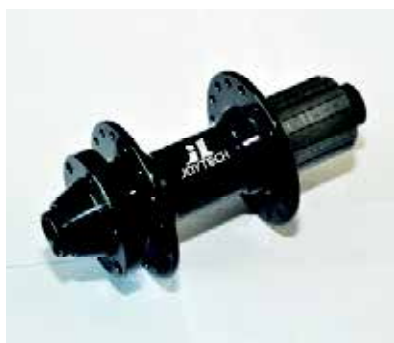
▲ Novatec's X12 loose ball bearing hub comes in 12X142 mm. It is ideal for more economically priced mountain bikes, and low assembly costs keep the hub affordable.
