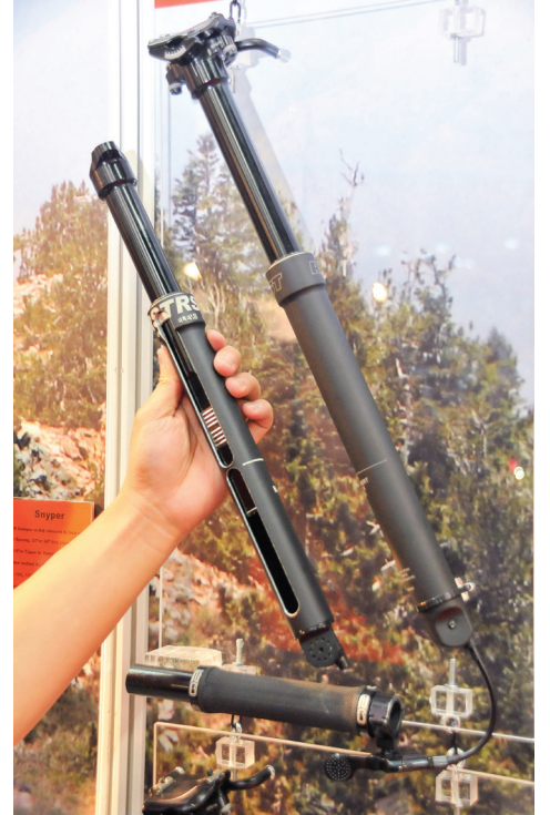
▲ RST's Elev8 dropper seatpost is designed with an internal rectangular shaft that rolls on needle bearings to prevent twisting. The Elev8 comes in lengths of 80, 100, 125 and 155 mm travel.
