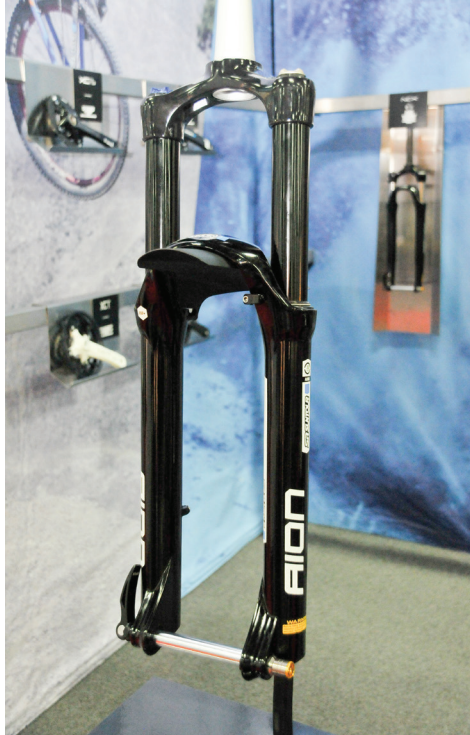
▲ SR Suntour upgraded its Aion product line to 27.5+, with an inner diameter of 35mm for better rigidity.
