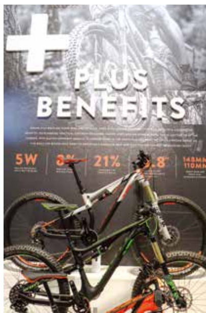
▲ The new "+"—"Plus"—concept promoted by Scott involves the use of 2.8" tires and a slightly lower tire pressure (1-1.2Bar) to achieve better steering and rolling performance. Scott has also introduced 11 Plus models to provide consumers with ample choice.
