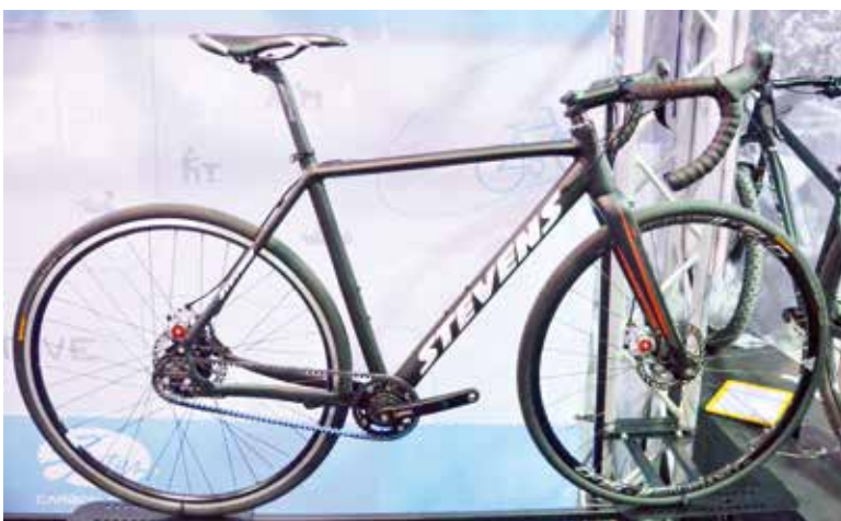
▲Stevens' gravel bike has a belt transmission system.
