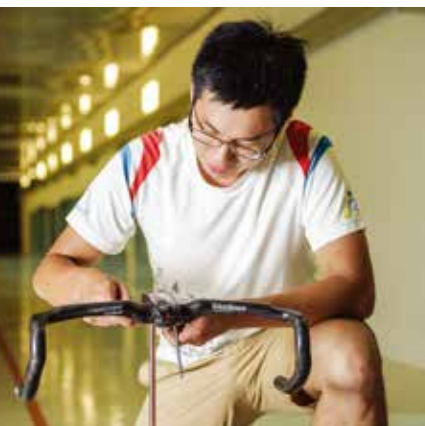
▲ After handlebars were installed on a jig, a special device was used to measure the drag coefficient; the handlebars were also mounted on a rotating platform in order to obtain the drag coefficient at different angles.
