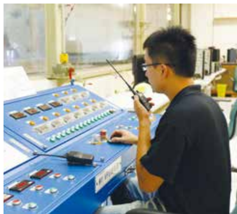
▲ Wind tunnel laboratory personnel at the Architecture & Building Research Institute, MOI adjust wind speed in the wind tunnel control room.
