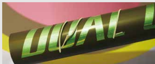
▲ HR tape showing heat deformation after use.
