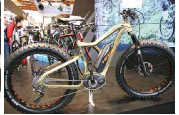
▲ Haibike decided to enclose the drive unit with the frame.
