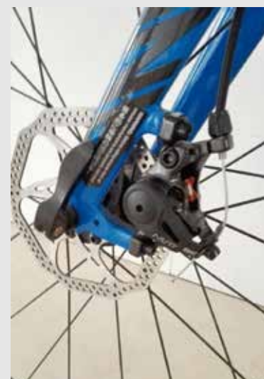
▲ The S-2, Lanxi Jieke's new dual-actuated disc brake for road bikes.
