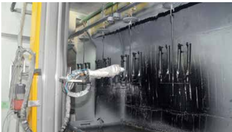
▲An all-new painting line featuring rotating cup spray-painting equipment seeks to shorten the painting process, boost efficiency, and keep management costs within reasonable limits.
